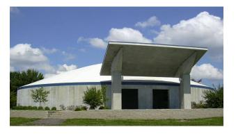
The unique shape of the shelter's curved surfaces force the wind around the shelter on all sides  $% \label{eq:curved_shelt}$
