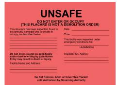
Buildings damaged by a disaster that pose an imminent safety threat under expected loads or likely conditions, like future rainfall or aftershocks, are posted with a red placard reading UNSAFE. A larger area beyond the property lines may need to be protected and should be indicated as such on the form. Alternatively, a relatively sound building may be tagged red due to a falling hazard or an adjacent unsafe structure or condition.
